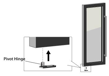
9. Install the door to the left hinge side by tightening the Pivot Hinge with the 2 screws.
